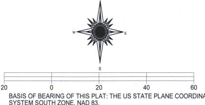
BASIS OF BEARING OF THIS PLAT: THE US STATE PLANE COORDINATE SYSTEM SOUTH ZONE, NAD 83.
